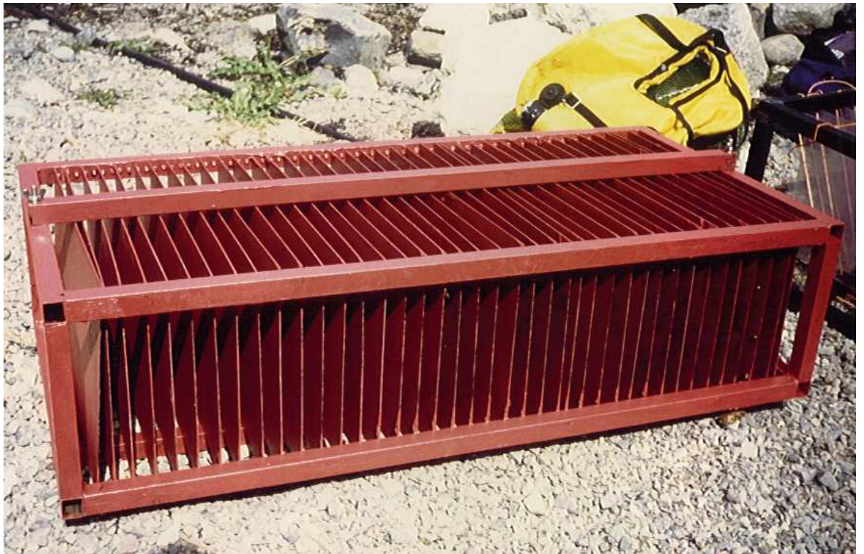
Figure 3.2 The completed array structure with antifoul-coated plates inserted.
